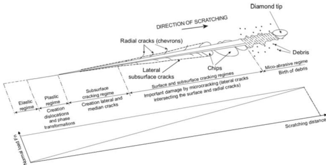
Figure 2. Model scratching test typical of vitreous materials proposed by Le Hou rou et al. (2003). Source: Wasmer, *et al.* (2005)
