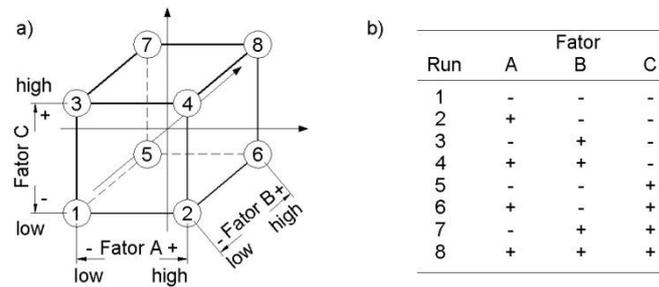
Figure 3. a) geometric view of a  $2^3$  design b) design matrix of a  $2^3$  experiment
