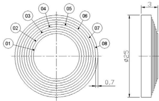
Figure 8. Views of the machined sample
