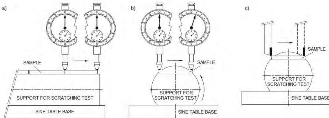
Figure 5. Execution of the nano-scratching tests: a) tilting procedure along the transversal direction; b) leveling procedure along the longitudinal direction; c) displacement of the tool
