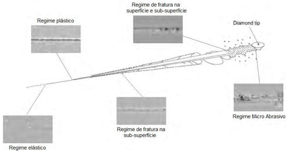
Figure 6. Comparison between the images found for ZERODUR<sup>®</sup> nano-scratching test and the model presented by Le Houérou *et al.* (2003)
