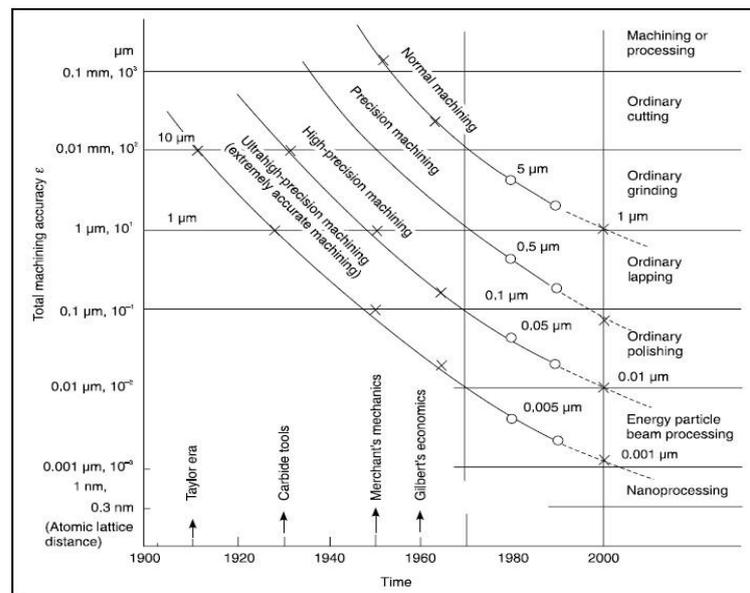
Figure 1. Evolution of the machining processes, machines and tolerances. Source: Venkatesh and Izman (2007)
