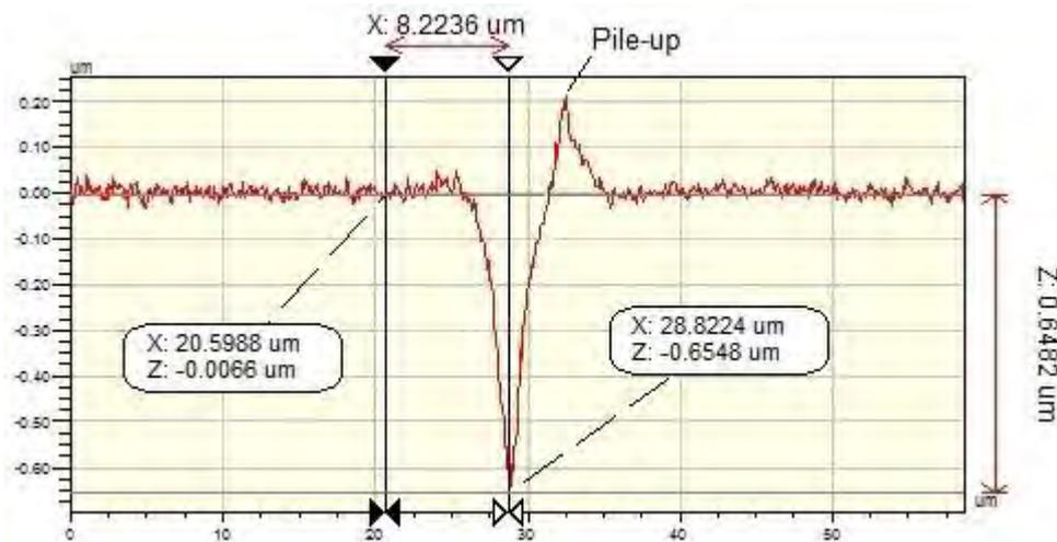
Figure 4. Analysis of the depth of the indentation using an interferometric optical profiler. The profile shows a pile-up of the material with approximately 1/3 of the total indentation depth
