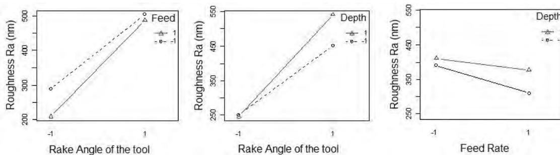
Figure 10. Plots of the interaction effects  $E_{AB}$ ,  $E_{AC}$  and  $E_{BC}$  respectively
