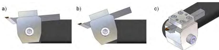
Figure 7. Adjustable tool fixture: a) for 5°, b) for 20°, c) isometric view.
