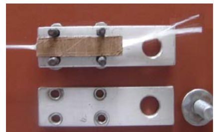
Figure 6. Terminal system used in the long term creep tests.
