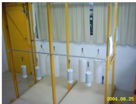
Figure 4. Creep test device using dead weights.
