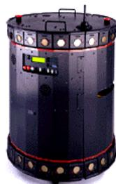
Figure 1. The Nomad XR4000 mobile robot
