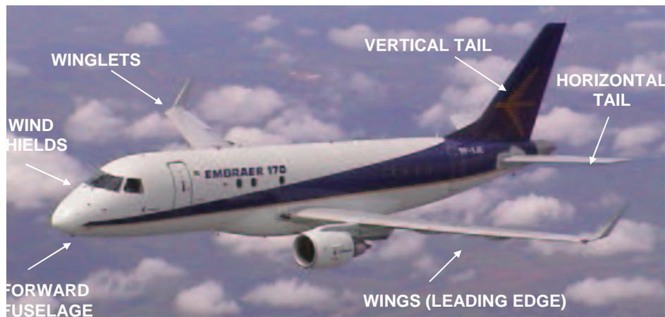
Figure 8. Regions in an aircraft that have to be tested against impact of birds.
