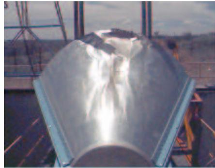
Figure 7. An aircraft nose after being impacted by a testing bird.
