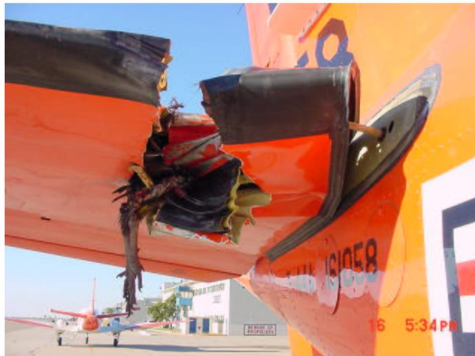
Figure 5. Impact of a bird on the rear wing of an aircraft.
