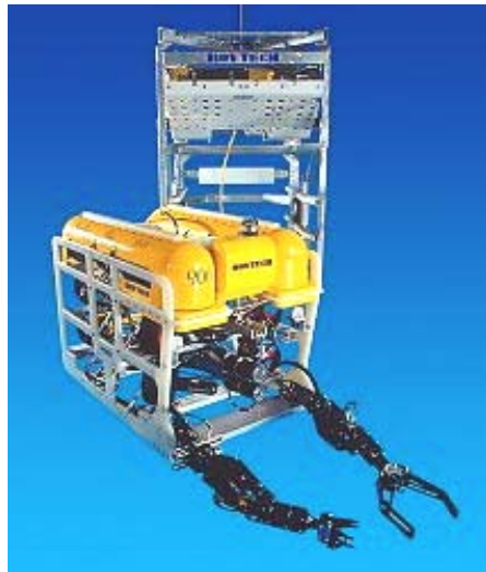
Fig. 1. ROV with manipulator and grabber arms (Seaeye, 2003).
