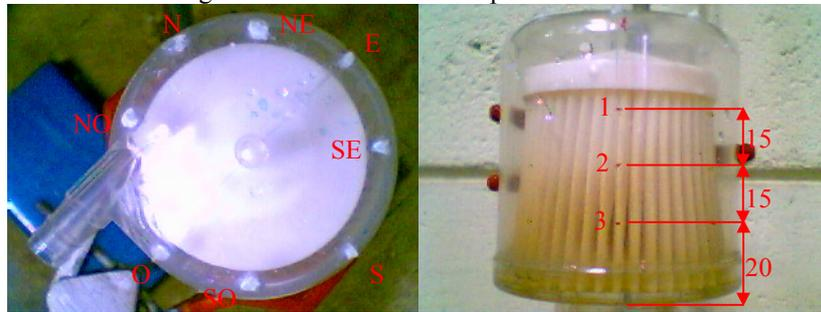
Figure 5 – Injection points and levels
