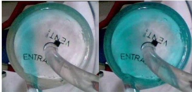
Figure 6 – Flow visualization at the upper part of the filter at two different instants of time
