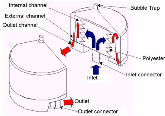
Figure 1. Schematic view of the filter
