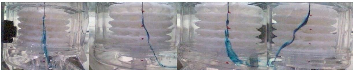
Figure 7 – Flow visualization in the external channel, in planes O, N, E and S, respectively.
