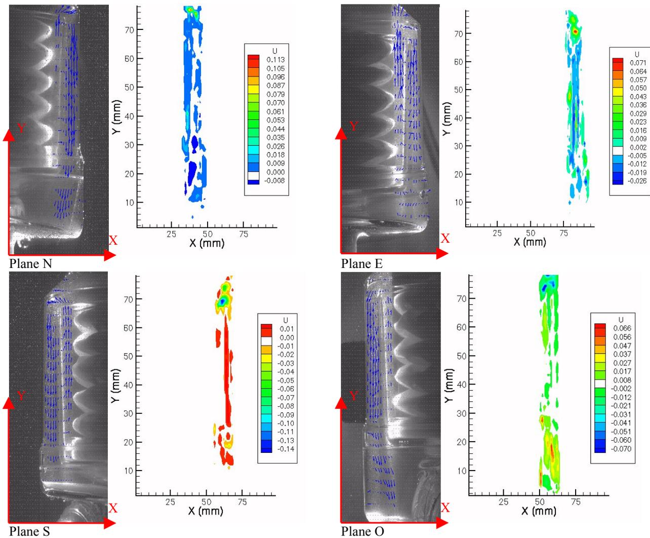
Figure 9 – Radial velocity in m/s
