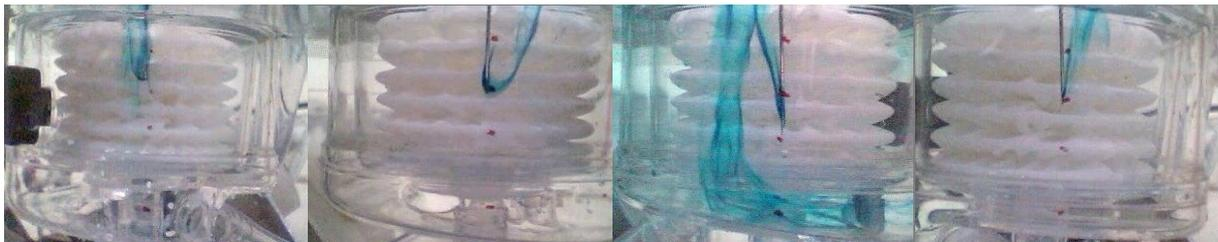
Figure 6 – Flow visualization in the internal channel
