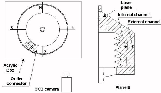
Figure 3 – Coordinate systems and measurements planes
