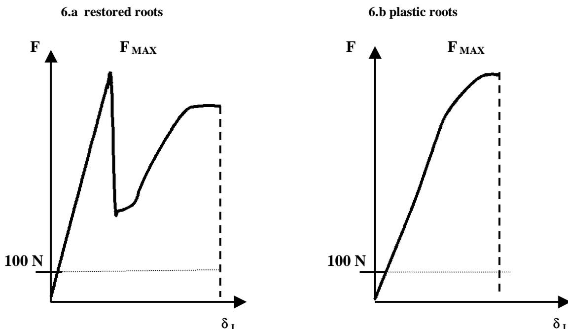
Figure 6 – Force – displacement diagrams of the test results of the ten specimens with restored **natural roots** (6.a), and the twelve specimens endowed with analogous **plastic roots**.
