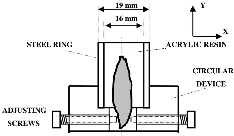
Figure 3 – Cross section of the circular device used to centralize the teeth.
