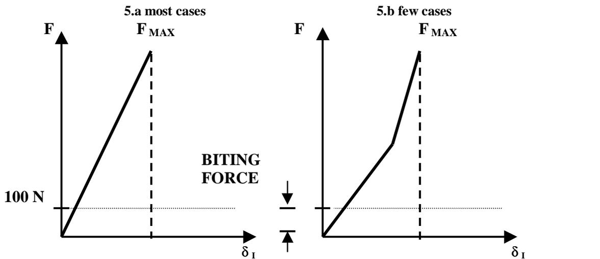
Figure 5 – Force – displacement diagrams of the test results of the eight **natural roots** with crown preparation.
