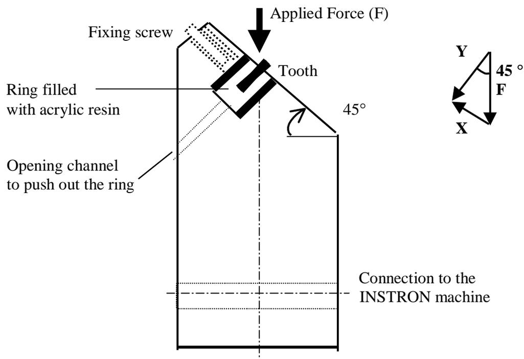
Figure 2 – Lateral view of the device developed for the destructive evaluation of the teeth.
