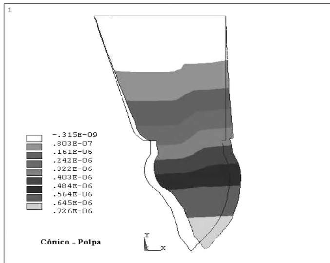
Figure 7 – Distribution of displacements along X [m] for the 2-D analysis concerned with the natural teeth.
