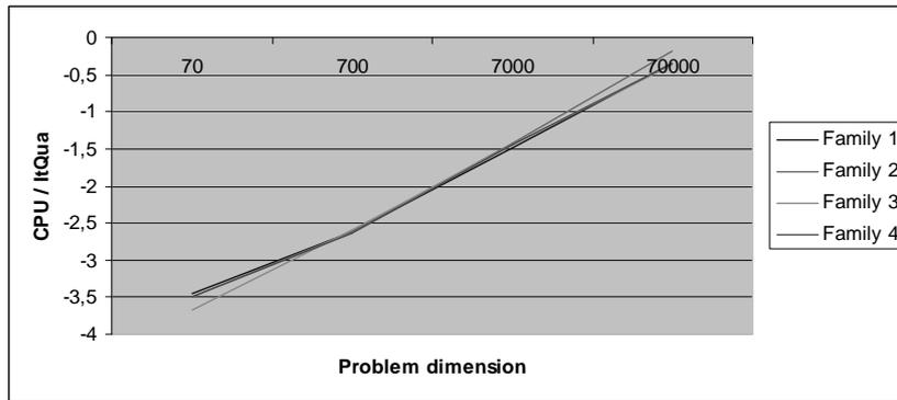
Figure 1. Log-log plot of problem dimension against the rate CPU/ItQua for each test family of Bertseka's control problems.
