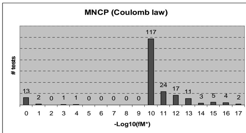
Figure 2. Objective function value ( $f_M^*$ ) distribution of problem (2) for contact problem with original Coulomb friction law.
