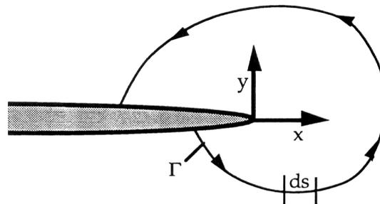
Figure 2. Arbitrary path around crack tip.
