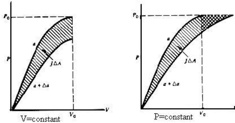
Figure 3. Graph for J Integral evaluation tests.
