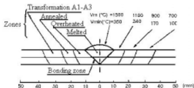
Figure 1. Different regions on a welded joint resultant from the imposed thermal cycle.
