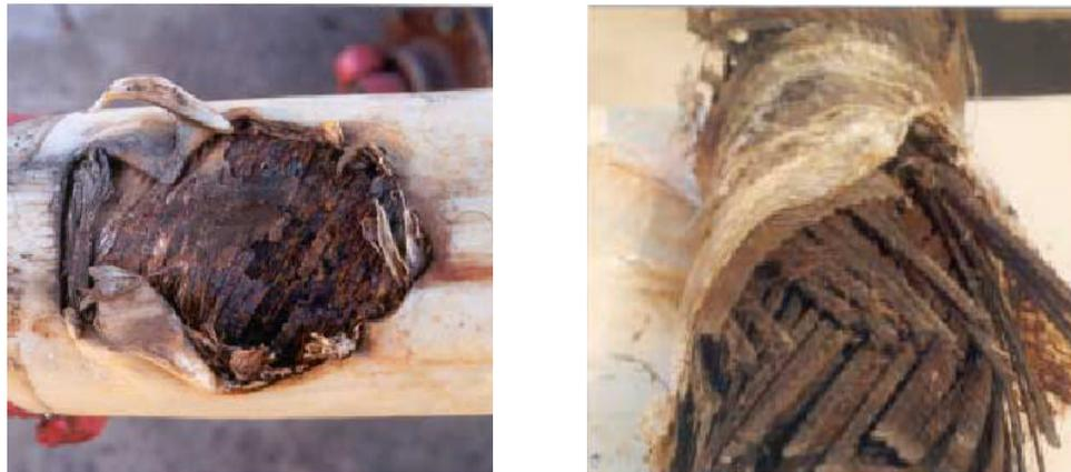
Figure 2. Effect of the corrosion in the internal structure of a flexible line due to fissures in the polymeric outer sheath.
