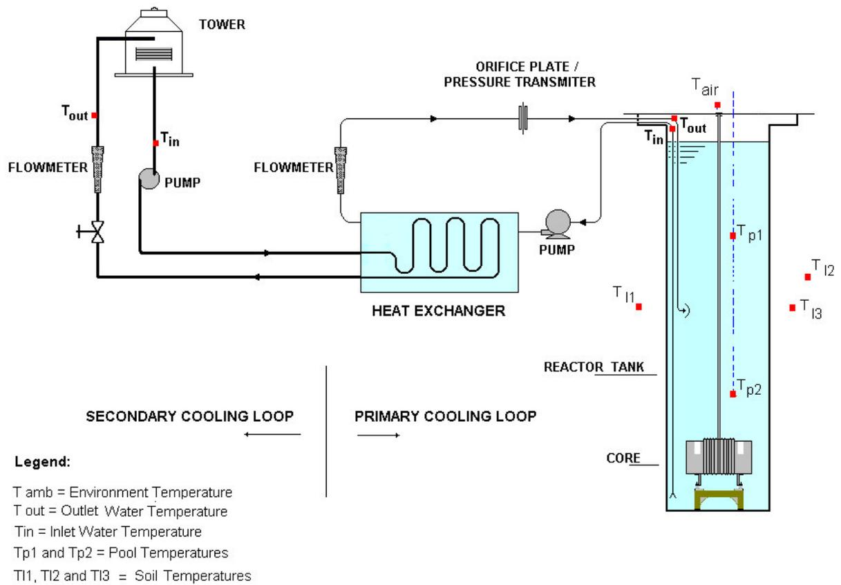
Figure 1. The 250 kW TRIGA MARK I IPR-R1 Research Reactor Cooling System with the used instrumentation.
