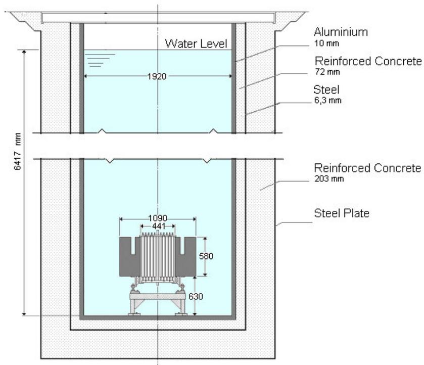
Figure 2. The TRIGA MARK I – IPR-R1 reactor pool.
