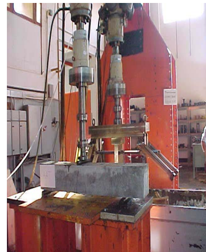
Figure 4. (a) Load x displacement plot measured and (b) Fatigue test experimental setup.
