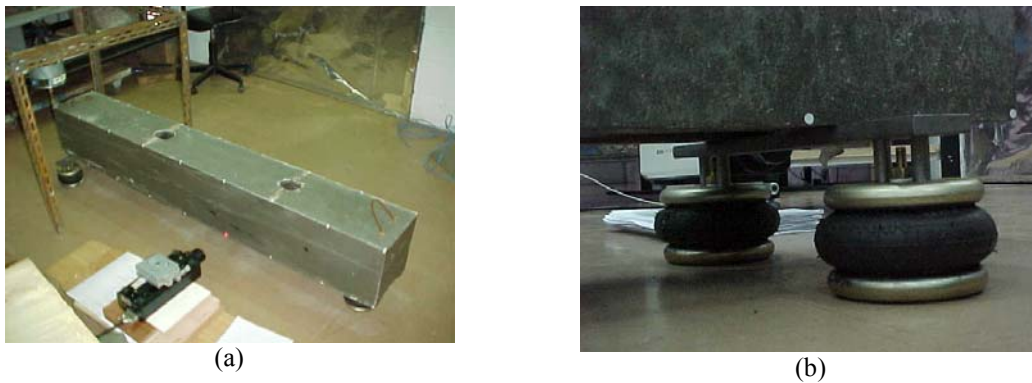
Figure 5. Dynamic experimental setup: (a) general view and (b) pneumatic springs detail.
