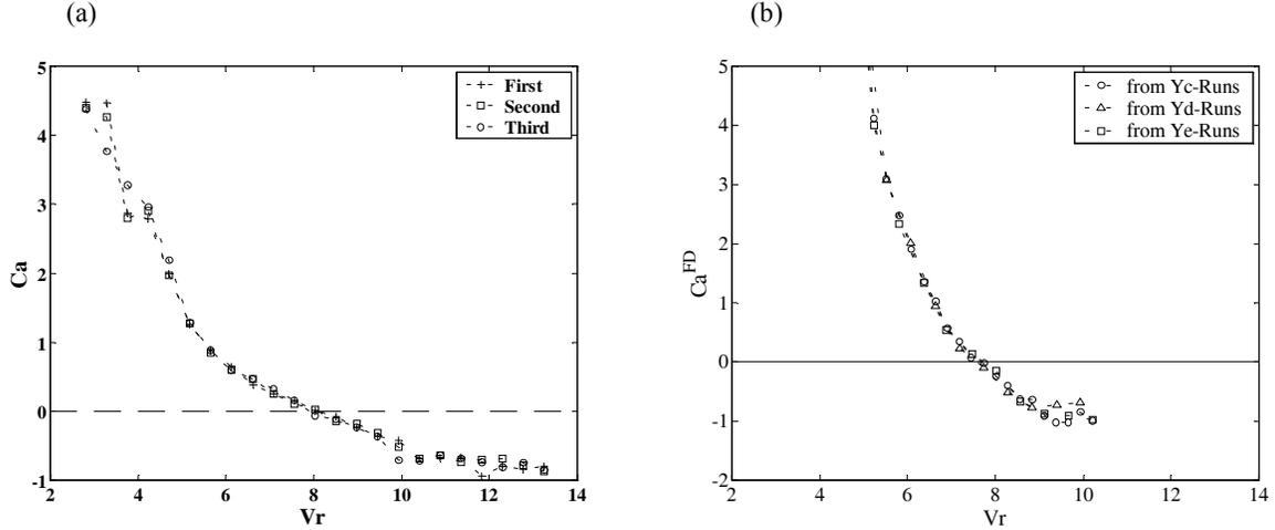
Figure 1. Added mass coefficient versus reduced velocity, concerning the first eigen-frequency in the cross-wise direction. (a) From time domain analysis: Vikestad, Vandiver and Larsen (2000) (b) From frequency domain: Fujarra and Pesce (2002a). In both cases, oscillation in the stream-wise direction is constrained.
