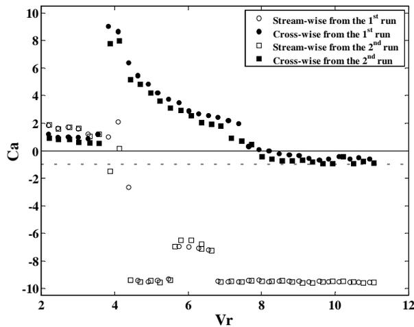
Figure 6. Stream-wise and cross-wise added mass versus reduced velocity concerning the first eigen frequency in the cross-wise direction. Rigid cylinder is free to oscillate in both directions (x and y).
