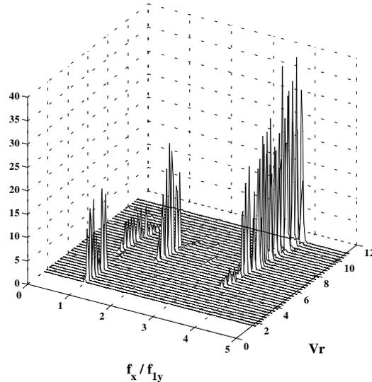
Figure 4. Waterfall of x-acceleration power spectra (stream-wise) shows the coexistence of different sub-harmonic orders at the lock-in peak.
