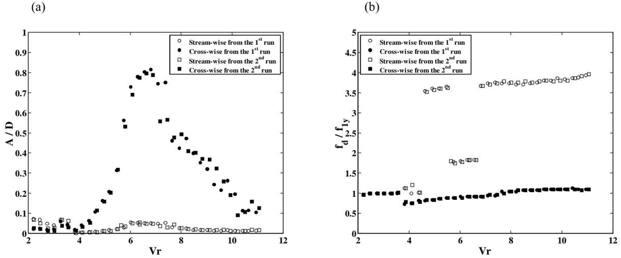
Figure 3. Response of a rigid cylinder elastically supported with two-degrees of freedom (x and y) and low structural damping, Pesce and Fujarra (2002). (a) Non-dimensional amplitudes in the cross-wise direction ( $\blacksquare$  and  $\bullet$ ) and in the stream-wise direction ( $\square$  and  $\circ$ ). (b) Respective non-dimensional dominant frequency responses.
