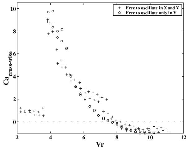
Figure 5. Cross-wise added mass versus reduced velocity. (+) Rigid cylinder is free to oscillate in both directions (x and y). (o) Rigid cylinder is free to oscillate only in cross-wise direction (y).
