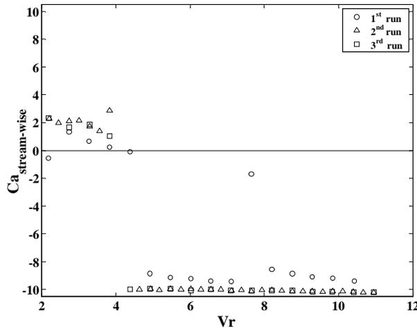
Figure 7. Stream-wise added mass versus reduced velocity. Rigid cylinder is free to oscillate only in stream-wise direction (x).
