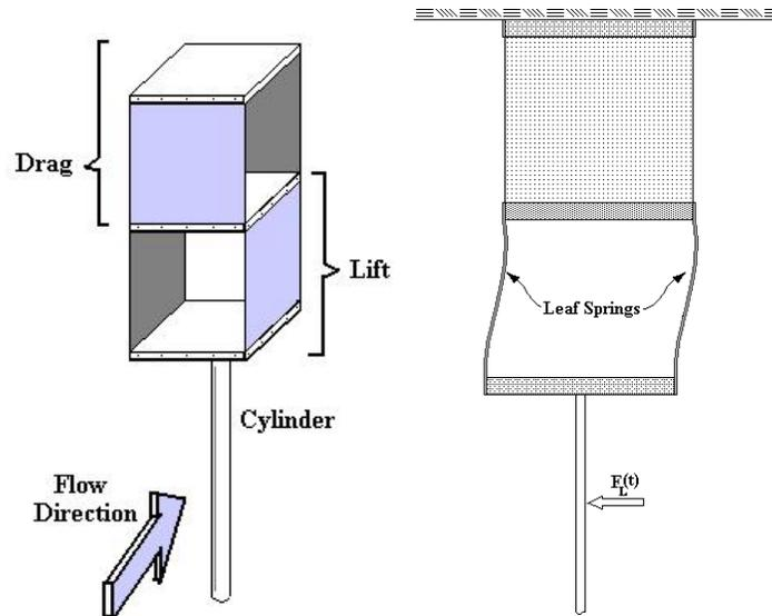
Figure 2. Sketch of the elastic support: a device with two degrees-of-freedom (x and y) and low structural damping.
