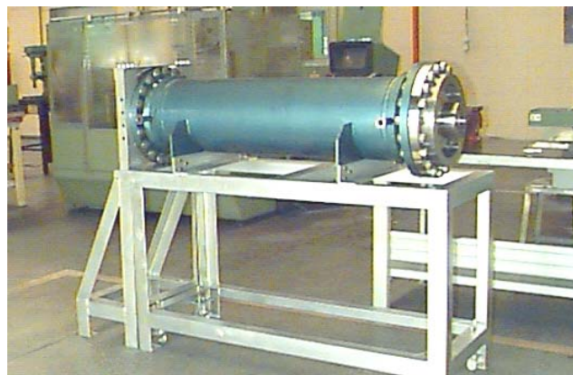
Figure 5: The new vitiated air generator (VAG)
