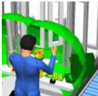
Figure 9: Proximity favored best reach of steel plates – they are inside green area.
