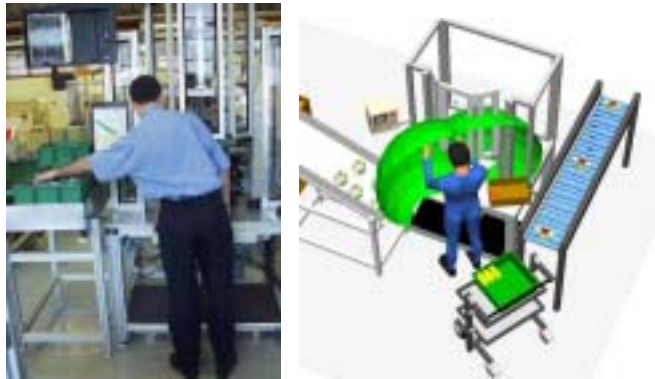
Figure 4: Back view of the operator – the green area represents the limit of operator reach
