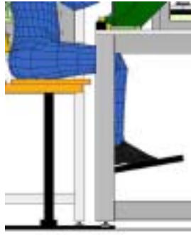
Figure 10: Elimination of the stand bar, increasing space for legs.
