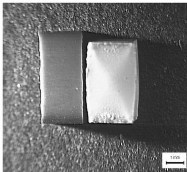
Figure 3. External surface morphology of specimens: (left) – before creep tests; and (right) a specimen crept under a stress of 300 MPa at  $1300^\circ\text{C}$  (1573 K) characterized by a mixed tension and compression region.
