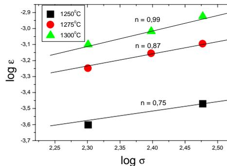
Figure 4. Stress dependencies of creep rate for hot-pressed  $\text{CRE}_2\text{O}_3/\text{Al}_2\text{O}_3$ -doped-  $\text{Si}_3\text{N}_4$  ceramic, under  $1250^\circ\text{C}$  ( $1523\text{K}$ ),  $1275^\circ\text{C}$  ( $1548\text{K}$ ) and  $1300^\circ\text{C}$  ( $1573\text{K}$ ).
