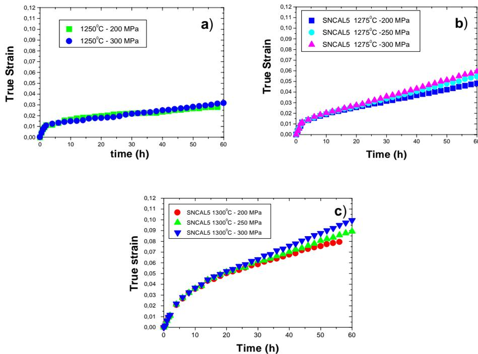
Figure 2. Creep curves of the hot-pressed silicon nitride specimens: a) at  $1250^\circ\text{C}$ ; b) at  $1275^\circ\text{C}$ ; c) at  $1300^\circ\text{C}$  (200 ~300MPa).
