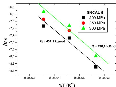
Figure 5. Temperature dependencies of creep rate for  $\text{Si}_3\text{N}_4$  ceramics under 200, 250 and 300 MPa stresses.
