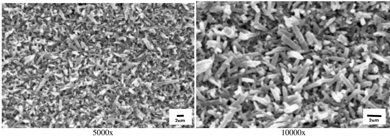
Figure 1. Microstructure of the hot-pressed creep specimens.
