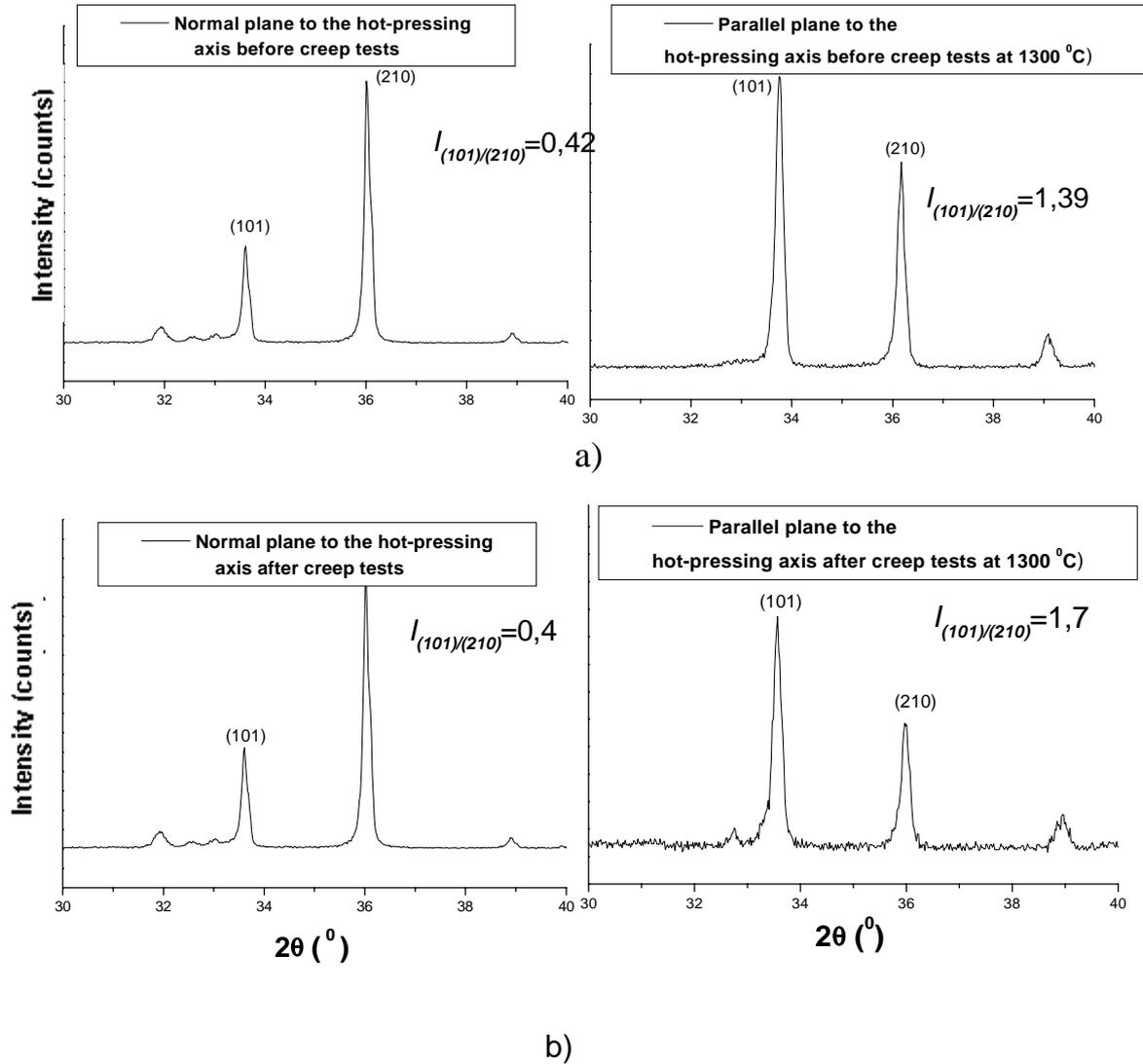
Figure 6. XRD patterns of specimens: a) before creep tests, in the perpendicular (normal) plane to the hot-pressing axis (N) and parallel plane to the hot-pressing axis (P); b) after creep tests at 1300°C and 300 MPa, in the (N) and (P) planes.
