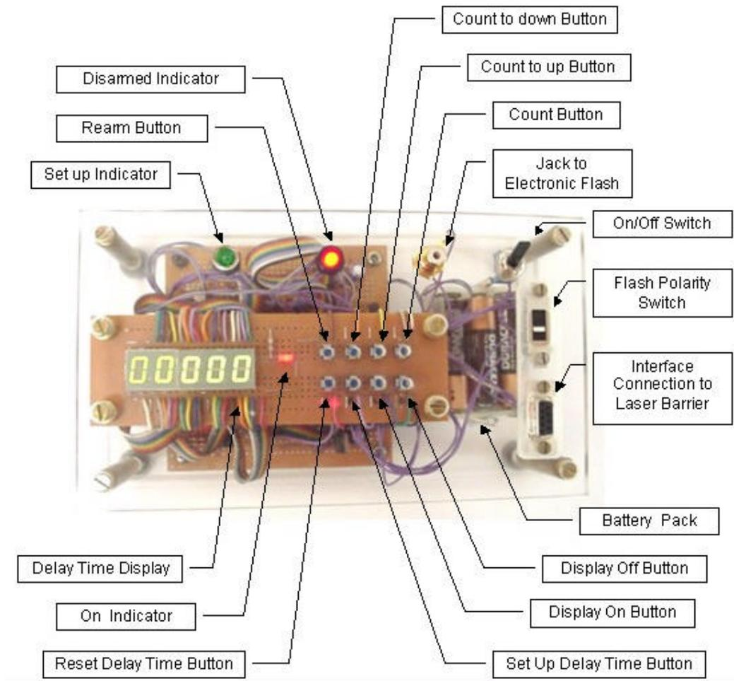
Figure 2. Front view of the developed digital electronic control device.
