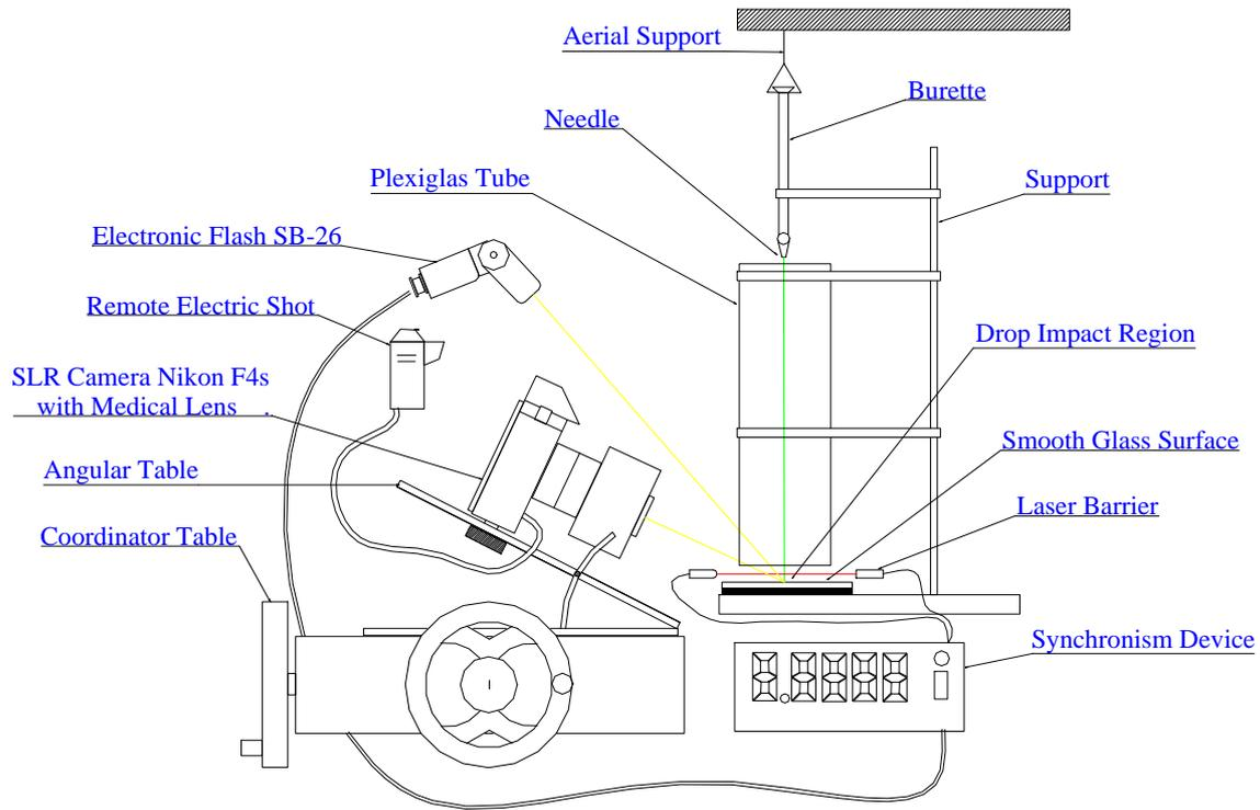
Figure 1. Experimental apparatus.
