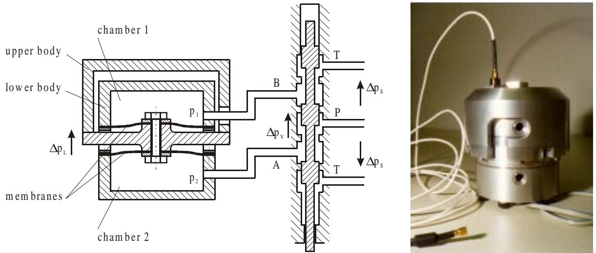
Figure 1- Sketch and prototype of the hydraulic actuator.
