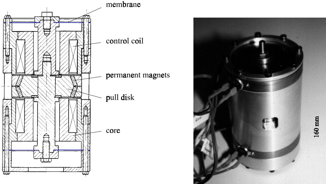
Figure 4- Sketch and prototype of the magnetic actuator.
