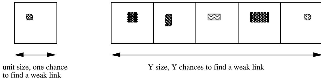
Figure 5 - Schematic showing how the statistical model works
