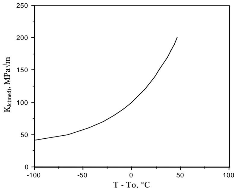
Figure 6 - Master Curve of  $K_{Jc(\text{med})}$  values in the transition
