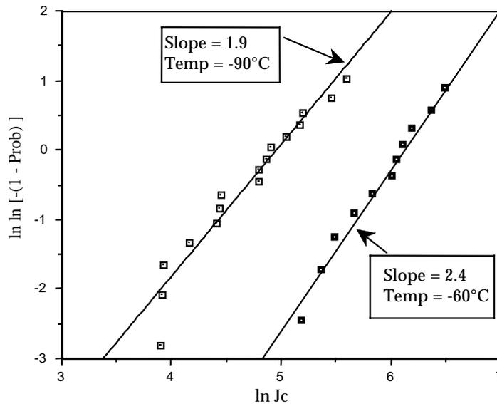
Figure 4 – Weibull plot for transition toughness of a steel at two temperatures
