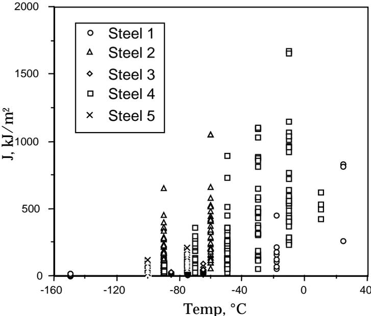
Figure 2 - Transition toughness results for five steels
