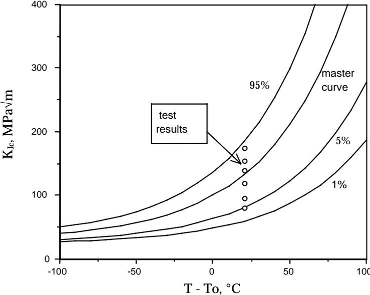
Figure 7 - Master Curve with tolerance bounds
