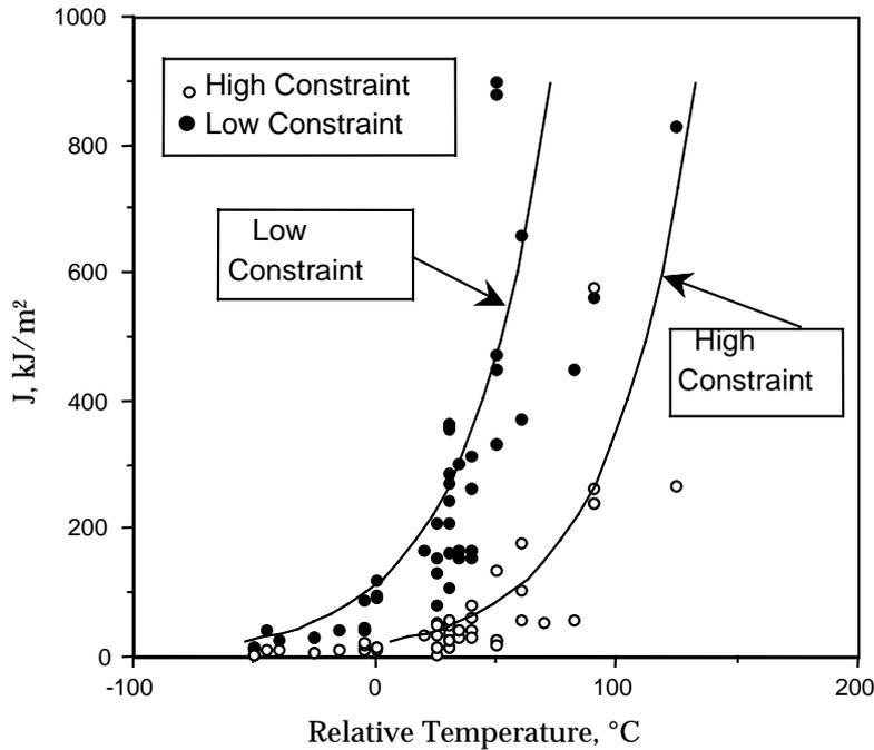
Figure 3 - Transition fracture toughness data with constraint trend lines
