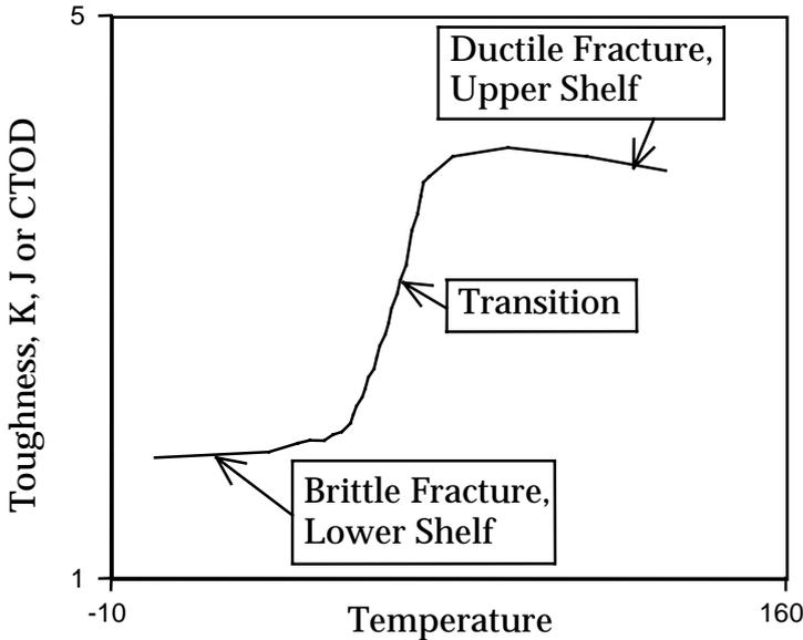
Figure 1 - Schematic showing region of transition fracture
