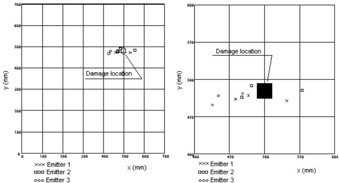
Figure 14: Damage localization resulting from the wavelet transform analysis.
