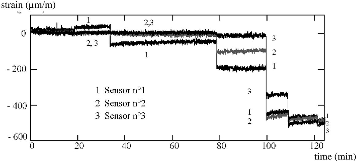
Figure 4: Strain measured by FBG sensors, resulting from successive impacts ( $E = 6, 8, 10, 12, 15, 18, \text{ and } 20 \text{ J}$  for respective values of time = 12, 18, 34, 78, 100, 108, and 122 min).
