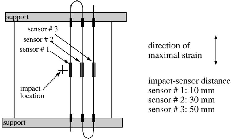
Figure 3: Integrated FBG sensor arrangement into a sandwich material coupon
