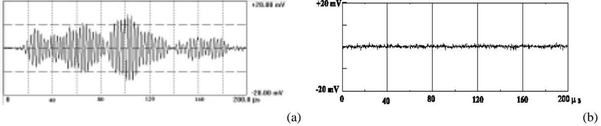
Figures 11: (a) Algebraic difference between signal obtained with damage and reference (no damage); (b) Difference between two reference signal
