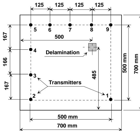
Figure 10: Experimental arrangement for acousto-ultrasonic detection
