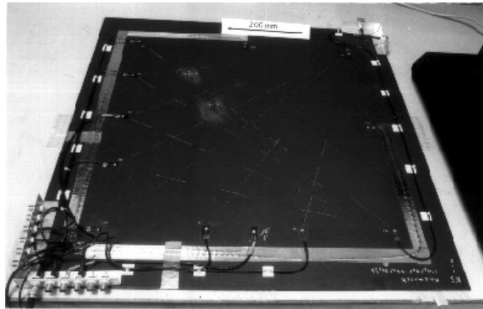
Figure 7: C/epoxy plate (700 mm × 700 mm) – *right* -, instrumented with miniaturized piezoelectric sensors - *left* -.
