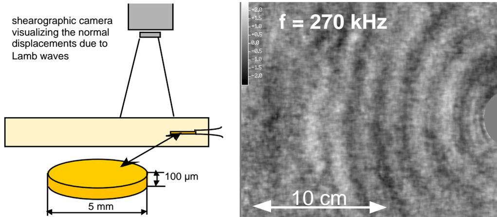
Figure 9: Visualization of the Lamb waves generated by a disc-shaped piezoelectric transducer embedded in a C/epoxy composite.
