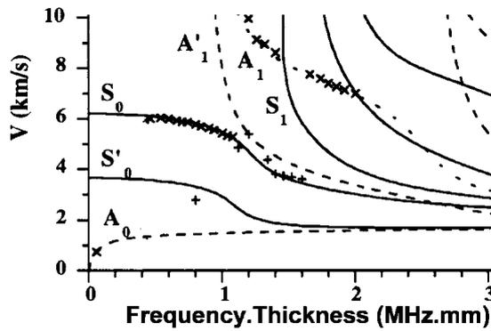
Figure 12: Dispersion diagram of a quasi-isotropic material
