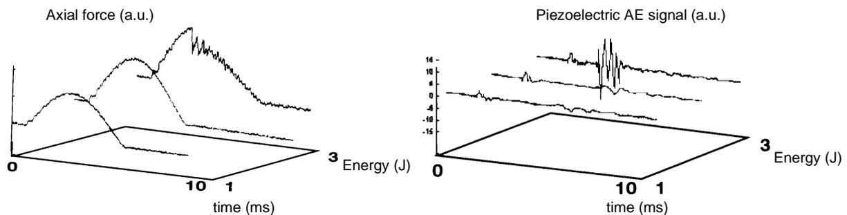
Figure 6: Damage threshold detection by piezoelectric transducers (high frequency vibrations apparition) correlated with the shape change of the force on the impactor head.
