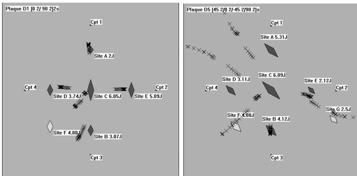
Figure 8: Localization of impacts calculated from piezoelectric sensor signals for different values of the parameters  $\xi$  and  $\lambda(x)$  in the case of coupons D1 (cross-ply) and D5 (quasi-isotropic), made of composite T300-914 C-epoxy, with dimensions: 500 x 500 x 2 mm.
