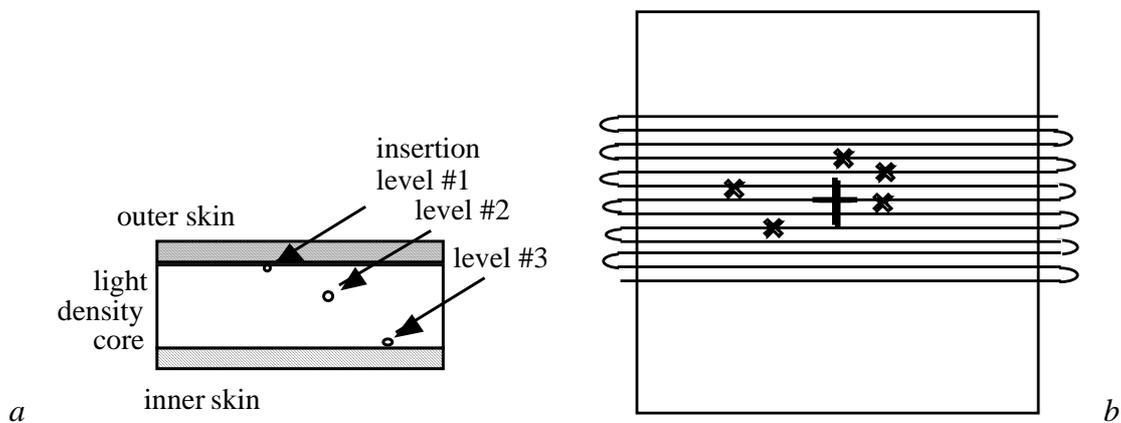
Figure 2: Coupon equipped with OTDR system: a) possible insertion levels for the fiber, b) fiber arrangement in the coupon, with the real 10 J impact site (+) and the defect locations derived from OTDR signals (x).
