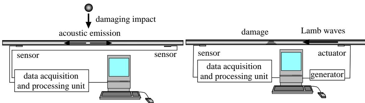
Figure 1: Possible use of a piezoelectric transducer network. *Left*: acoustic emission technique; *right*: acousto-ultrasonics, or Lamb waves based technique.
