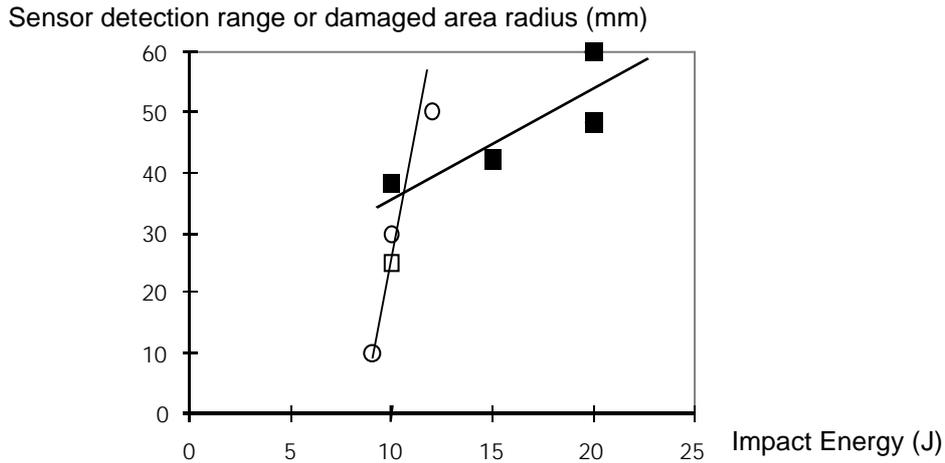
Figure 5: Comparison between OTDR (□) and FBG sensors (○) detection ranges to the best estimate of actual damaged area radius (◆).
