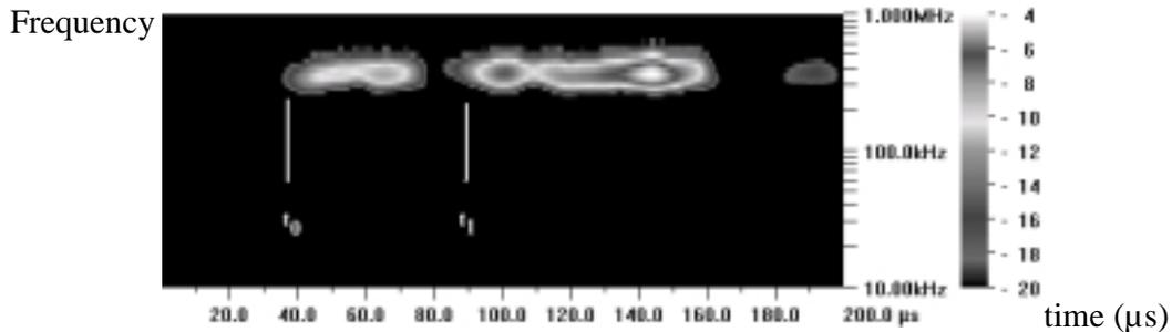
Figure 13: Time-frequency diagram of the differential signal for propagation path 2-7.
