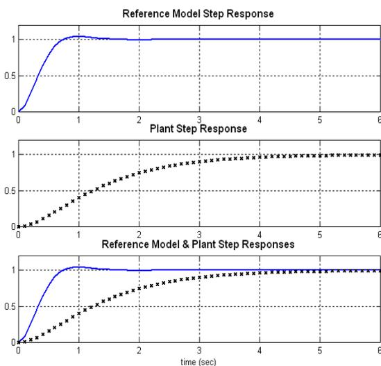
Figure 8a. Plant Open Loop Response for  $J=0.10$ .
