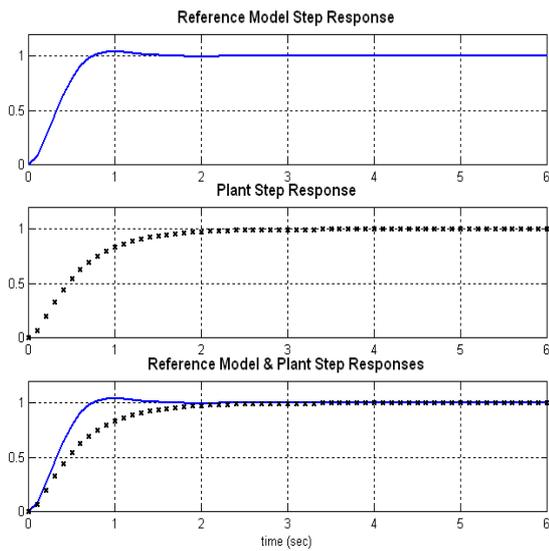
Figure 6a. Plant Open Loop Response for  $J=0.01$ .
