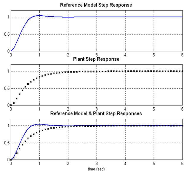
Figure 5. Reference Model Specification for Design Purposes.
