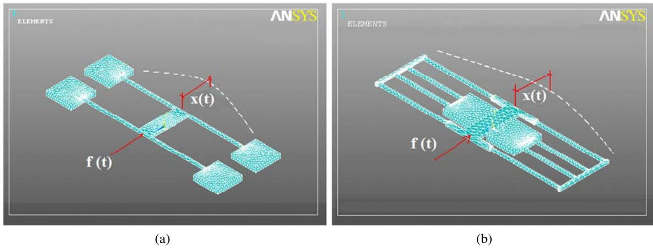
Figure 3. MEMS structures: (a) Double Bridge (b) Hinge
