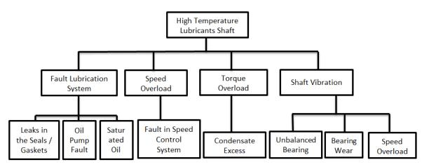
Figure 6. Suggested FTA for the top event "High Temperature Lubricants Shaft"
