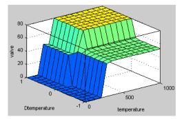
Figure 11. Surface generated by the fuzzy algorithm according to the fuzzy rules defined for the mitigation model.
