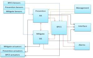
Figure 3. Control Architecture proposed for SIS Mitigation layer.
