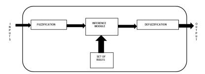
Figure 2. Schematic diagram of a Fuzzy Controller.
