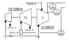
Figure 5. P&ID of a turbo compressor unit of the gas compression station.
