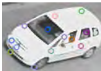
Figure 4: Keypoints detected for the reference object
