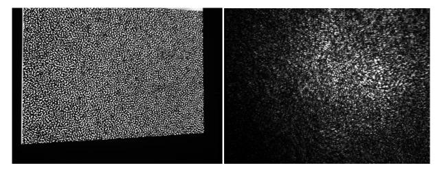
Figure 3: Acquired images from (a) band-limited random projection and (b) laser speckle projection.
