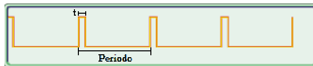
Figure 1 – Pulse Train example to be sent to the servo
