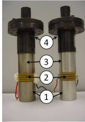
Figure 1. Langevin-type transducer. 1)Tail mass; 2) Piezoelectric disk stack; 3) Head mass; 4) mechanical amplifier
