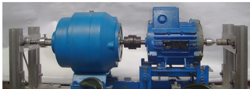
Figure 3. Industrial prototype of harmonic drive builds by Universidad Nacional de Colombia
