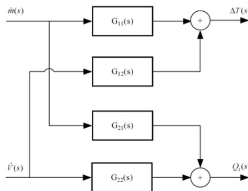
Figure 2. Evaporator Input-Output Variables and Cross Coupling.
