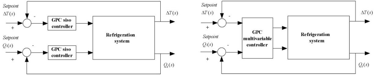
Figure 4. Multi Loop and Multivariable Controllers.
