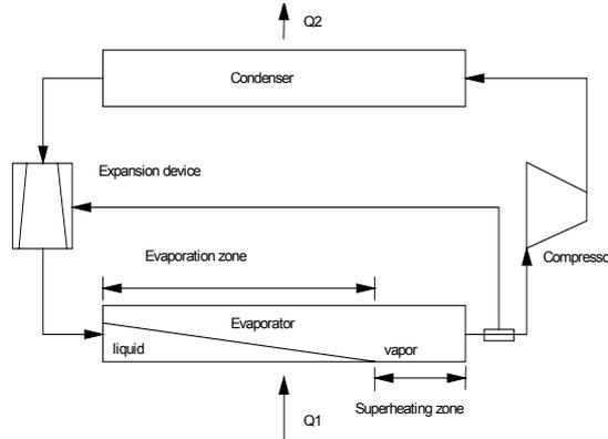
Figure 1. The Vapor Compression Based Refrigeration Cycle.
