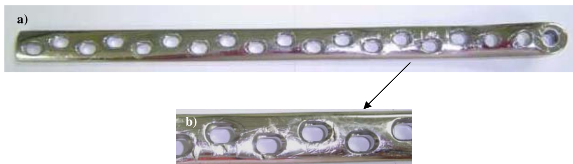
Figure 2. Photograph of the stainless steel plate after removal from the patient: (a) Overview of the entire piece; (b) Detail of the right side of the piece showing several risks.
