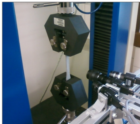
Figure 6: Cameras arrangement during the test
