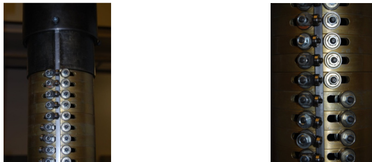
Figure 4: Rollers adjustment in experiments with the straight bars. Left: free to move radially; right: free to move laterally. The rollers to the extremities were adjusted to restrain both radial and lateral displacements.
