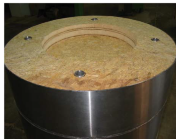
Figure 5: Bottom shock absorber partial assembling.
