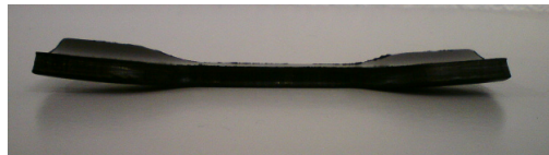
Figure 7: Detail of the specimen showing the curvature along the axial direction.
