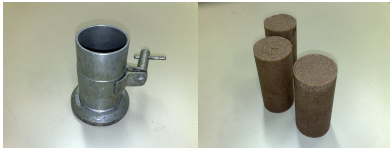
Figure 2: Compression test specimens.
