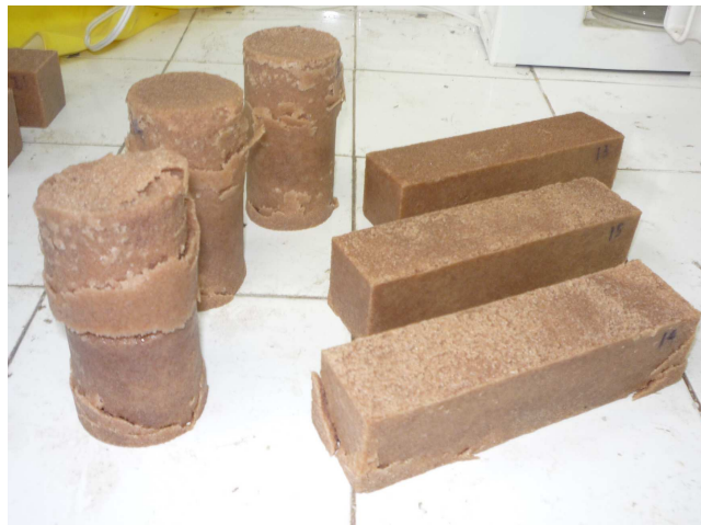
Figure 4: Specimens after lactic acid degradation.
