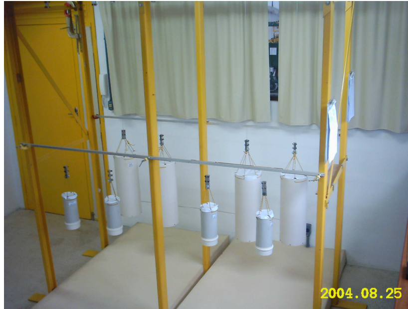
Figure 1: Dead weight creep test device
