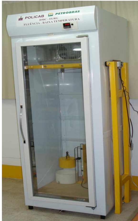
Figure 8: Creep cold equipment.
