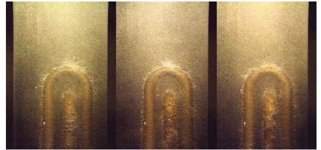
Figure 5. Saturated flow boiling.
