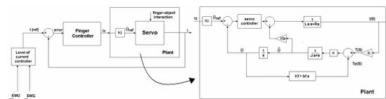
Figure 1: System plant and control architecture
