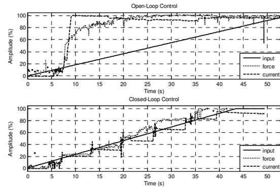
**Figure 3: Experimental results for force x current, (a) Open-Loop and (b) Closed-Loop.**
