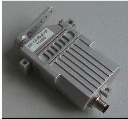
Figure 7 Selected actuator for the solar-powered UAV under study
