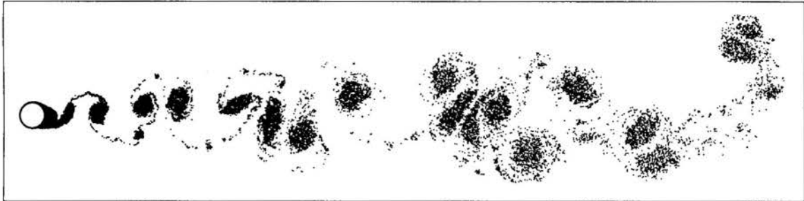
Figure 6 - Position of the wake vortices at t = 67.5 ; Re = 225000 , \alpha = 0.3 , N = 16 , \sigma_0 = \epsilon = 0.003 , \Delta t = 0.075 .
