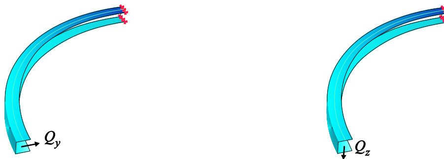
Figure 4 – Configuration of load cases in forced frequency analysis of a cantilever thin-walled curved U beam.
