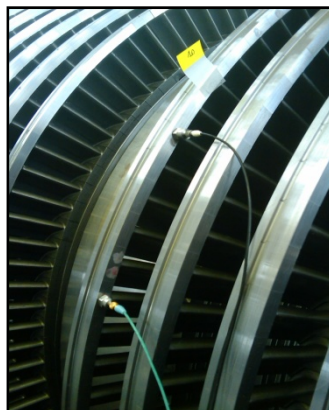
Figure 12 – Position of accelerometers during impulse tests
