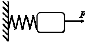
Figure 8. Mass spring test system.
