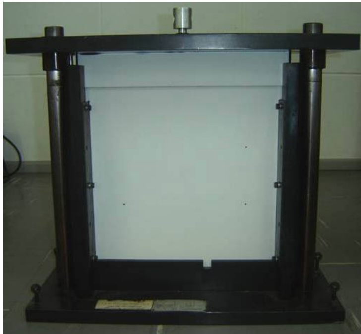
Figure 2 – Panel mounted in the test device.
