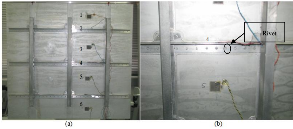
Figure 9. Aircraft panel: (a) 6 PZT patches bonded to the structure; (b) metallic rivet.
