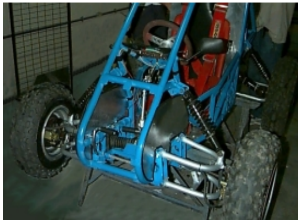
Figure 1. Mini-Baja vehicle front suspension detail. (2002 “B12C” CEFET/RJ team)
