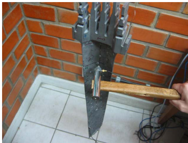
Figure 3. Experimental set for the modal testing of a single blade in a free-free condition
