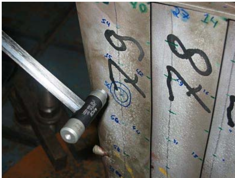
Figure 6. Experimental setup for the modal testing of a five blades group in a clamped-free condition, showing selected impact point.
