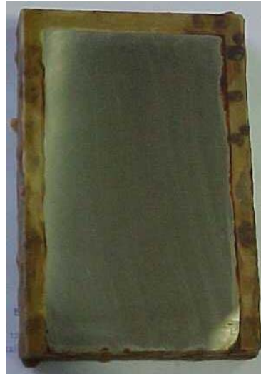
Figure 11. Salt spray test results, 200 \mu\text{m} thick after 750 hours.
