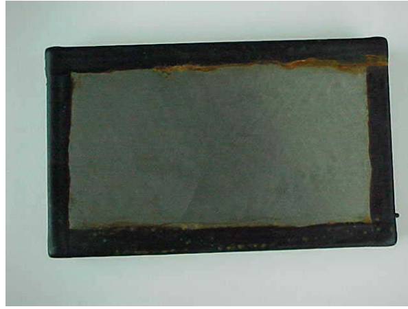
Figure 8. Salt spray test results, 150 \mu\text{m} thick after 750 hours.
