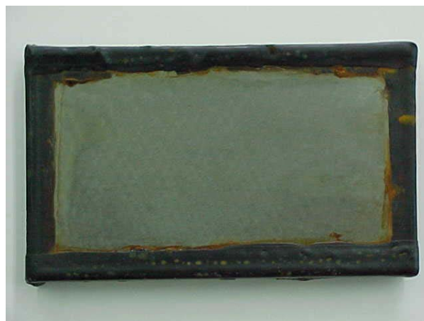
Figure 7. Salt spray test results, 100 μm thick after 750 hours.
