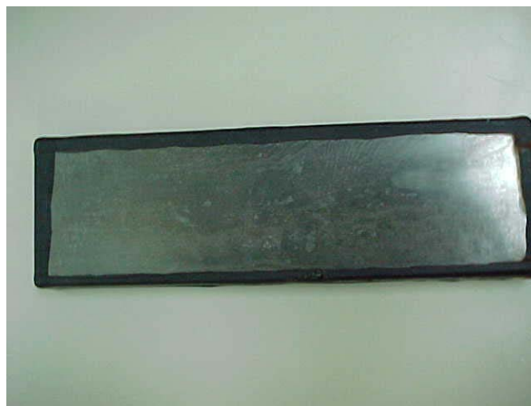
Figure 9. Salt spray test results, 200 \mu\text{m} thick after 750 hours.
