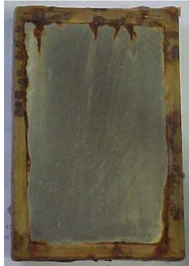
Figure 10. Salt spray test results, 150 \mu\text{m} thick after 750 hours.
