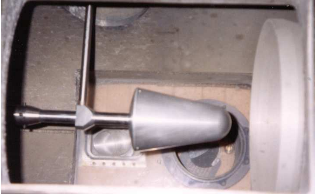
Figure 5: Ballistic re-entry vehicle SARA model (with the locations of pressure transducers).
