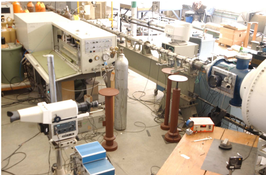
Fig. 3. IEAv Hypersonic Shock Tunnel test section and the CO 2 TEA laser heads.
