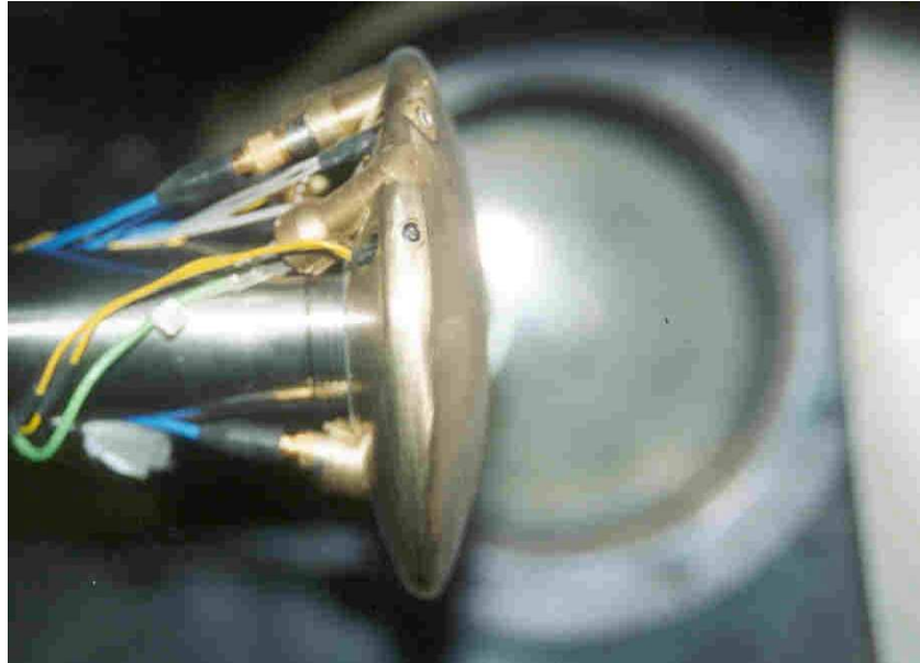
Fig. 4 Photograph of the instrumented Double Apollo Disc model.
