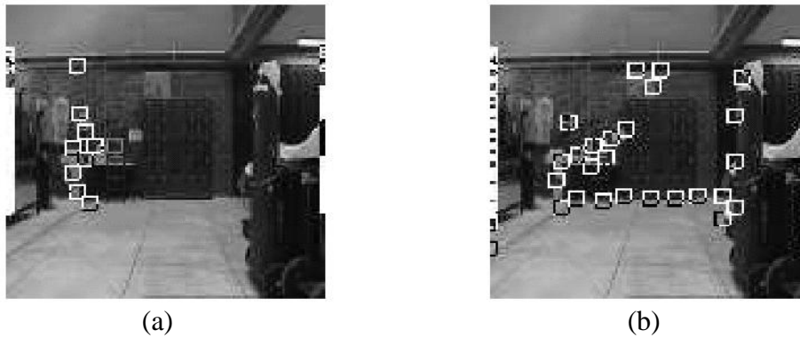
Figure 5. (a) Non-uniform and (b) uniform searching for feature points.
