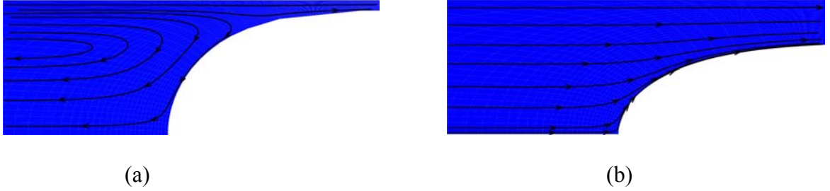
Figure 3. Newtonian flow field as a function of Ca . Figure (3a) shows the streamlines for Ca = 0.02 ( m < 0.5 ) and Fig. (3b) shows the streamlines for Ca = 1.00 ( m > 0.5 ).
