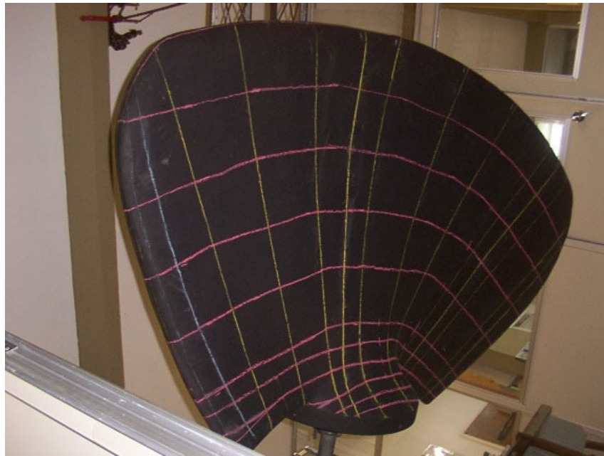
Figure 4 – Mapped lines on Kaplan turbine runner surface
