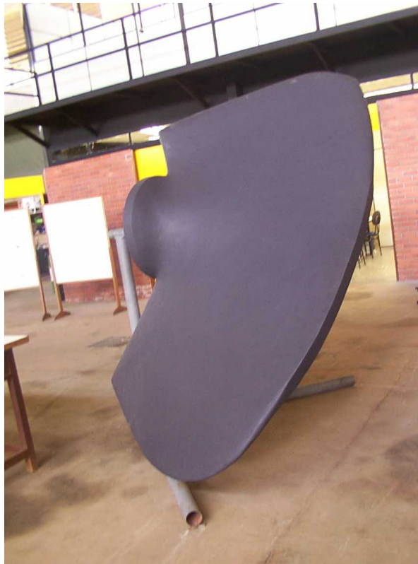
Figure 2 – Kaplan turbine runner prototype
