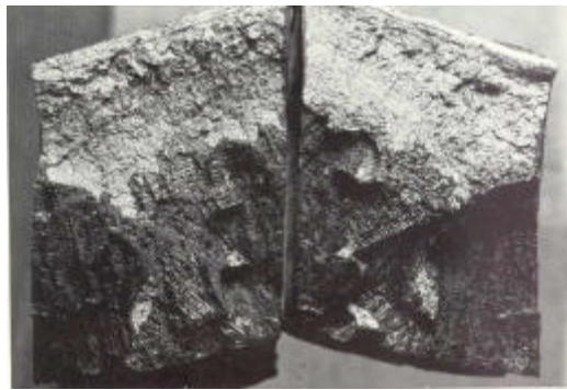
Figure 1. Cast Steel Part with a Hot Tear
