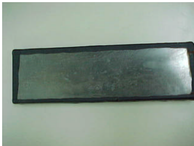
Figure 9. Salt spray test results, 200 \mu\text{m} thick after 504 hours.
