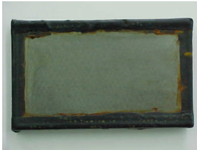
Figure 7. Salt spray test results, 100 \mu\text{m} thick after 504 hours.
