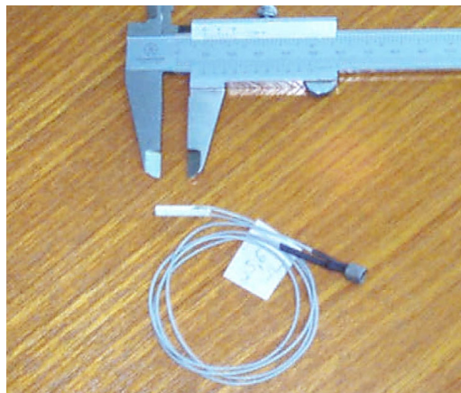
Figure 1: Thin-film platinum heat gage
