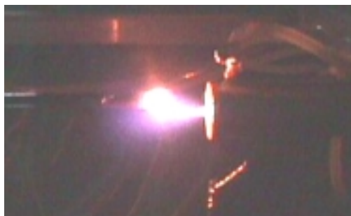
Fig. 13 – Photography of the plasma source in operation illustrating its capability to heat and to melt a titanium sample.
